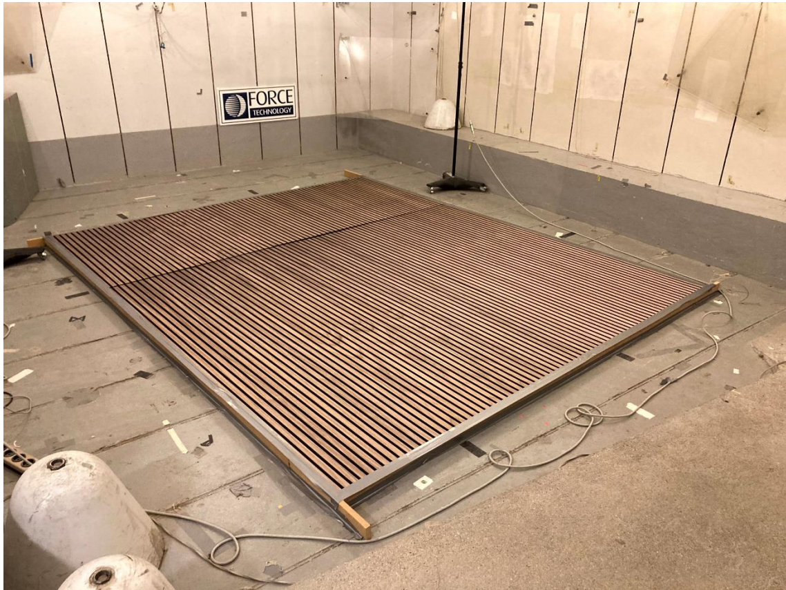
Figure 1 Acupanels Træ Panels mounted in the laboratory (Type E-65 mounting).
